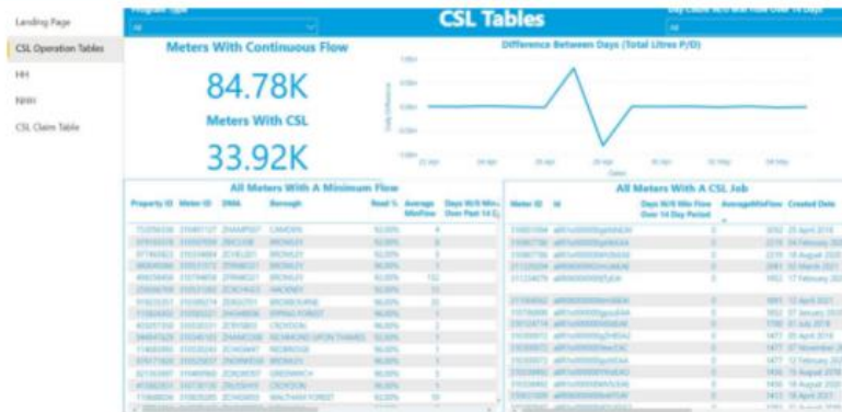
Smart Continuous Flow & Customer Side Leakage - Providing data from TWM and MDMS giving more insight into continuous flows per prop and jobs raised in TWM -
